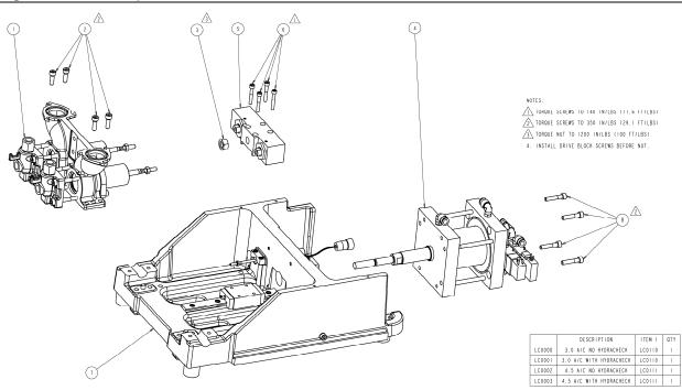
Figure 39: PR70 Base Frame to Air Cylinder, Pump and Drive Block Attachments
